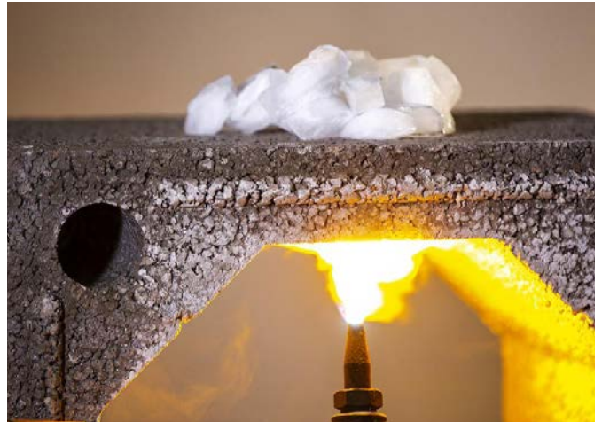
Pumice: is an excellent insulator, keeping flue gases warm while not transmitting heat to the outside.
