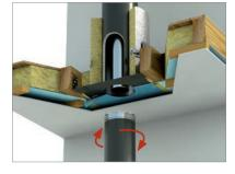
6. Insert lowering pipe into the ceiling box and lock it in place with a fast turn of the pipe. A twist-lock mechanism ensures the pipe remains in place.
