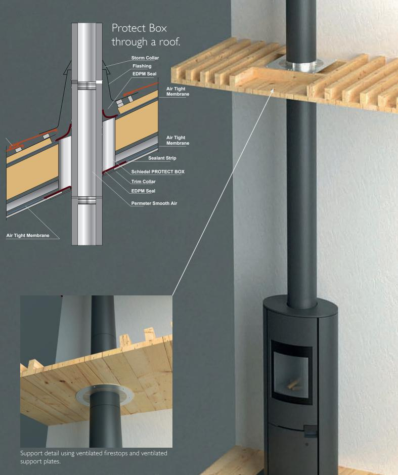
A ventilated firestop is used on the living room ceiling with a ventilated support plate at first floor level.
