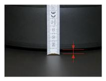
3. The outer case of the adapter should not be in direct contact with the top plate of the stove. There should be at least 5 mm clearance ensured.
