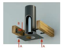
5. Position the ceiling box to the middle between the ceiling beams, flat with the lower side of the beams.
