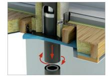
7. After installation of the stove, the stove adapter and chimney pipe (see pictures 1-3), release/unlock the lowering pipe by fast turn. Lower the pipe and push it down to fit both pipes together firmly.
