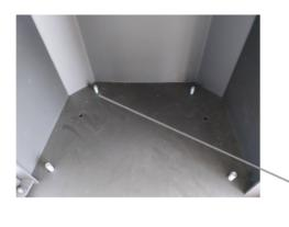
Adjusting screws for uneven floor (4x)
