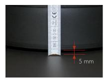
3. The outer case of the adapter should not be in direct contact with the top plate of the stove. There should be at least 5 mm clearance ensured.
