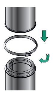
The joint is made by fitting the female end over the male end and engaging the joint system by rotating the component clockwise. A locking band is then fitted to secure the joint, as shown. The Vantage joint incorporates an eight barb twist lock coupler system to allow easy and rapid installation of the product.
