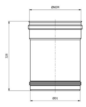
The 1-Piece ME Adjustable length is a lightweight and simple alternative to the existing ME 2 piece Adjustable Length, which allows for adjustment over smaller distances making it ideal for header/cascade systems.
