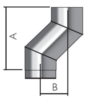
This component is used to provide a fixed offset of 100mm, by using two 45 degree bends.
