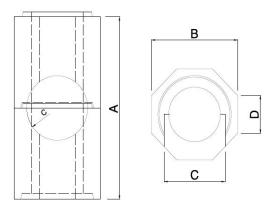
For DM Block Chimneys. Suitable for use in negative pressure (Dry Chimney) applications. CE Designation (T450 N1 D 3 G(00)
