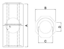
For DM Block Chimneys. Suitable for use in negative pressure (Dry Chimney) applications. CE Designation (T450 N1 D 3 G(00)
