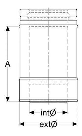
UK Plus Concentric flue system is a modular, high quality stainless steel concentric flue system for balanced flue applications.
