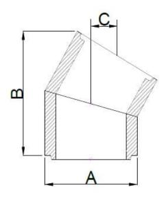
For lining masonry chimneys. Suitable for use in negative pressure (Dry Chimney) applications. CE Designation (T450 N2 D 3 G)
