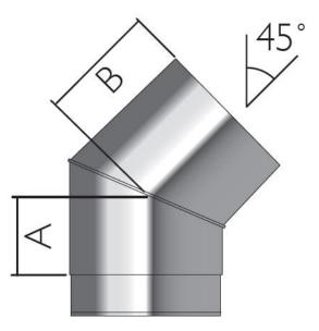
This item gives a fixed angle of 45 deg and when used in pairs gives a 45 deg offset in the connecting flue pipe. It can also be used in conjunction with a 135 Tee. Suitable for use in negative pressure (N1) applications.
