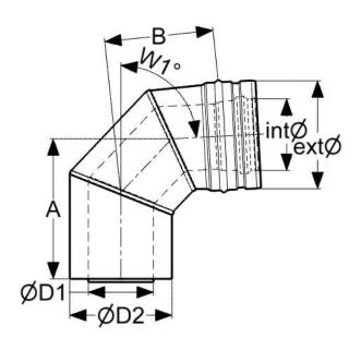
UK Plus Concentric flue system is a modular, high quality stainless steel concentric flue system for balanced flue applications.
