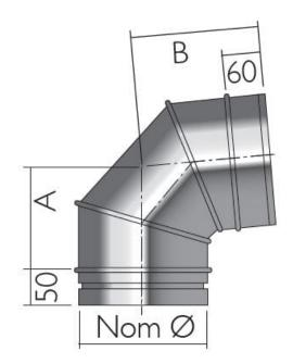
This item gives a fixed angle of 87° providing a slope. Suitable for use without any gaskets in negative pressure (N1) applications. By adding a lip seal gasket to the male end of the liner it can be used on positive pressure applications (P1).
