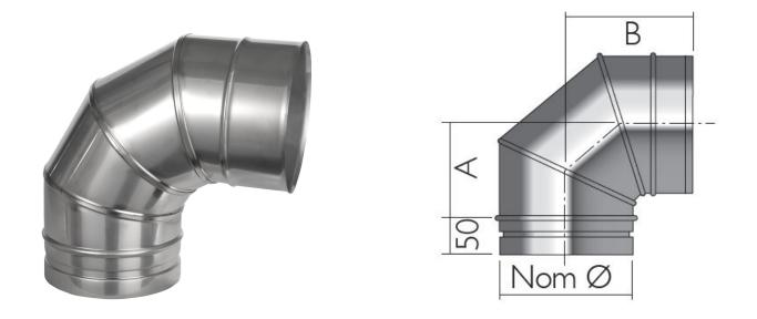
This item gives a fixed angle of 90°. Suitable for use without any gaskets in negative pressure (N1) applications. By adding a lip seal gasket to the male end of the liner it can be used on positive pressure applications (P1).
