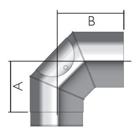
This item gives a fixed angle of  $90 \rightarrow$ . Suitable for use in negative pressure (N1) applications. The door, which is fixed in place by two Avdels, can be removed to allow for Inspection and cleaning on a connecting flue pipe application.
