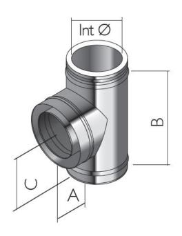
93 Deg Tee - ICS Tees. ICS is converted into ICS Plus by adding a lip seal to each component with a male form on the liner. This creates a twin wall insulated chimney system designed for the new generation of condensing gas and oil appliances, with continuous operating temperatures up to  $200^{\circ}$ C, short firing up to  $250^{\circ}$ C, and positive pressure up to  $200^{\circ}$ Da at the appliance outlet.
