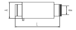
Absorption Silencer 25 dB (all welded) - MFSIA1 is part of our Silencers range for our Schiedel MF system, which is a modular twin wall insulated flue/chimney system, made of stainless steel, with a sealing ring.
