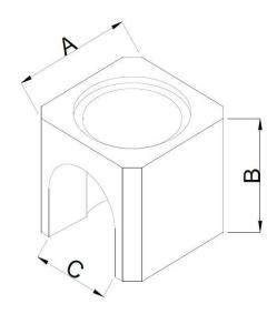
For providing sweeping access. Suitable for use in negative pressure (Dry Chimney) applications. CE Designation (T450 N2 D 3 G)
