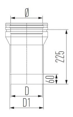
Adaptor double-double - MFADD is part of our Starting components / adaptors, Twin Wall range for our Schiedel MF system, which is a modular twin wall insulated flue/chimney system, made of stainless steel, with a sealing ring.
