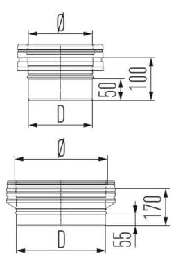
Adaptor - MFA is part of our Starting components / adaptors, Twin Wall range for our Schiedel MF system, which is a modular twin wall insulated flue/chimney system, made of stainless steel, with a sealing ring.
