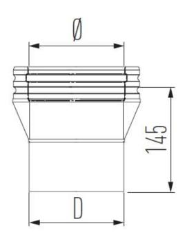
Adaptor smooth and tapered - MFAGT is part of our Starting components / adaptors, Twin Wall range for our Schiedel MF system, which is a modular twin wall insulated flue/chimney system, made of stainless steel, with a sealing ring.
