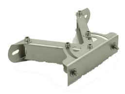
Adjustable distance block 75-175 mm for MFMB - MFMBAH299 is part of our Support components range for our Schiedel MF system, which is a modular twin wall insulated flue/chimney system, made of stainless steel, with a sealing ring.
