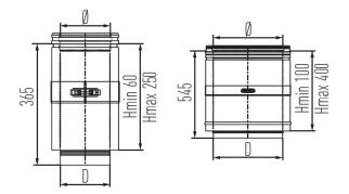
Adjustable length - MFPP is part of our Pipes range for our Schiedel MF system, which is a modular twin wall insulated flue/chimney system, made of stainless steel, with a sealing ring.
