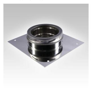
The Anchor Plate is used when commencing an installation with a fire chest, or when extending an existing brick or masonry chimney stack, an anchor plate must be used. The plate should be pushed into the opening of the fire chest with the plate resting on the bed of fire cement.
