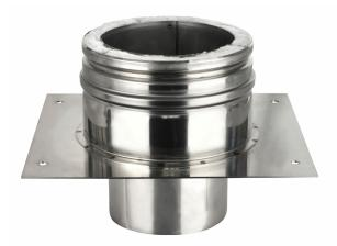
Anchor Plate - ICS Starting Components. ICS is converted into ICS Plus by adding a lip seal to each component with a male form on the liner. This creates a twin wall insulated chimney system designed for the new generation of condensing gas and oil appliances, with continuous operating temperatures up to 200°C, short firing up to 250°C, and positive pressure up to 200pa at the appliance outlet.
