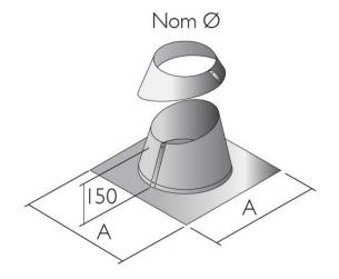
This item is manufactured with a malleable aluminium base and is used to provide a water tight flashing around the chimney as it passes through a roof pitched between 0-45 degrees. It is provided as a kit together with a stainless steel storm collar and a tube of silicon sealant.
