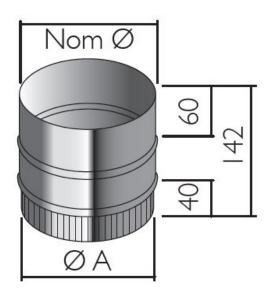
The item is used as an appliance connector and starts the connection from the appliance to the flue.
