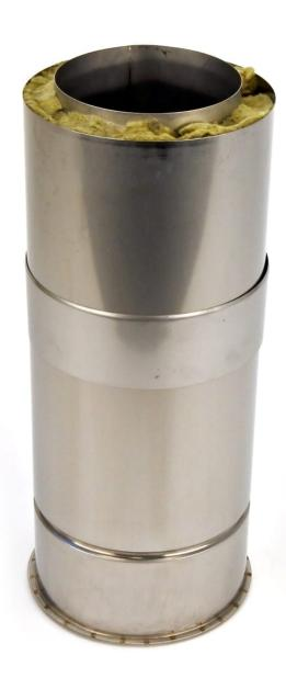
Ceiling /wall connector - MFPR is part of our Support components range for our Schiedel MF system, which is a modular twin wall insulated flue/chimney system, made of stainless steel, with a sealing ring.
