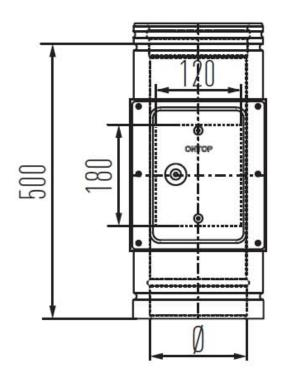
Clean out door - MFTR is part of our Pipes range for our Schiedel MF system, which is a modular twin wall insulated flue/chimney system, made of stainless steel, with a sealing ring.
