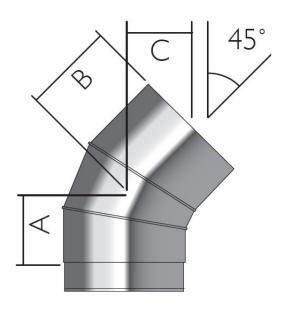
This item gives adjustable angle in range. 0°-45°. Suitable for use in negative pressure (N1) applications.
