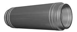
Combination silencer 25 dB (all welded) - MFSIC1 is part of our Silencers range for our Schiedel MF system, which is a modular twin wall insulated flue/chimney system, made of stainless steel, with a sealing ring.
