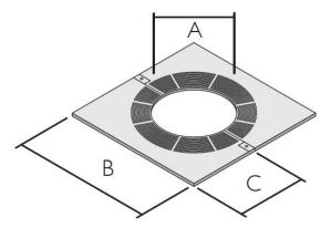
The ventilated firestop plate air to be circulated, preventing excessive heat build up in this area.
