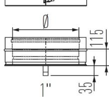
Condensate collector with drain - MFRBK is part of our Pipes range for our Schiedel MF system, which is a modular twin wall insulated flue/chimney system, made of stainless steel, with a sealing ring.
