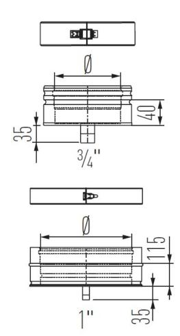
Condensate collector with drain - MFRBK is part of our Pipes range for our Schiedel MF system, which is a modular twin wall insulated flue/chimney system, made of stainless steel, with a sealing ring.
