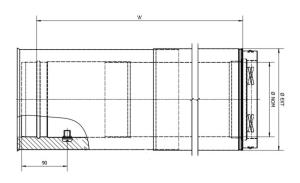
The new ICID DW Adjustable Starter Section now incorporates a dedicated test point on its liner, combining both connection to the appliance and a test point into one part. This will be introduced alongside the existing DW Adjustable Starter Section, giving customers a further option when connecting to their appliance using ICID.
