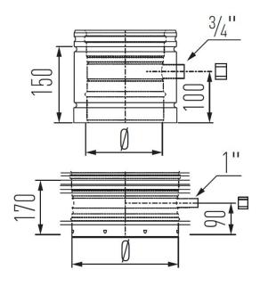
Drain (horizontal) / Probe length - MFEM is part of our Pipes range for our Schiedel MF system, which is a modular twin wall insulated flue/chimney system, made of stainless steel, with a sealing ring.
