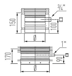
Drain vertical - MFEMC is part of our Pipes range for our Schiedel MF system, which is a modular twin wall insulated flue/chimney system, made of stainless steel, with a sealing ring.
