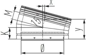
Elbow 15 Degree - MFB15 is part of our Bends range for our Schiedel MF system, which is a modular twin wall insulated flue/chimney system, made of stainless steel, with a sealing ring.
