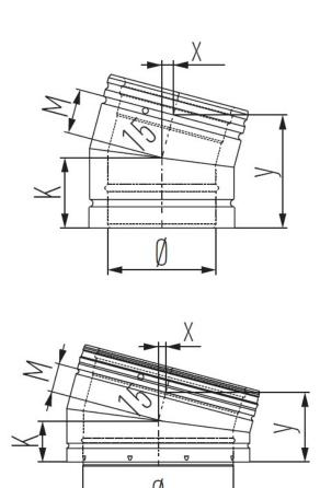
Elbow 15 Degree - MFB15 is part of our Bends range for our Schiedel MF system, which is a modular twin wall insulated flue/chimney system, made of stainless steel, with a sealing ring.
