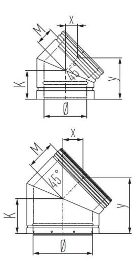
Elbow 45 Degree - MFB45 is part of our Bends range for our Schiedel MF system, which is a modular twin wall insulated flue/chimney system, made of stainless steel, with a sealing ring.
