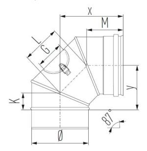
Elbow 87 Degree + inspect.cover - MEBI 87 is part of the Schiedel ME range, which has a number of applications and advantages.
