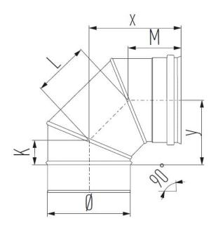
Elbow 90 Degree - MEB 90 is part of the Schiedel ME range, which has a number of applications and advantages.
