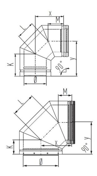
Elbow 90 Degree - MFB90 is part of our Bends range for our Schiedel MF system, which is a modular twin wall insulated flue/chimney system, made of stainless steel, with a sealing ring.
