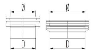
Increasing adaptor (D to be specified on order) - MFA00 is part of our Starting components / adaptors, Twin Wall range for our Schiedel MF system, which is a modular twin wall insulated flue/chimney system, made of stainless steel, with a sealing ring.
