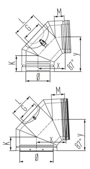
Inspection elbow 87 Degree - MFBI87 is part of our Bends range for our Schiedel MF system, which is a modular twin wall insulated flue/chimney system, made of stainless steel, with a sealing ring.
