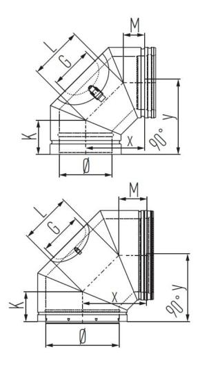
Inspection elbow 90 Degree - MFBI90 is part of our Bends range for our Schiedel MF system, which is a modular twin wall insulated flue/chimney system, made of stainless steel, with a sealing ring.
