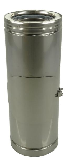
Inspection element for solid fuels - MFIH is part of our Pipes range for our Schiedel MF system, which is a modular twin wall insulated flue/chimney system, made of stainless steel, with a sealing ring.
