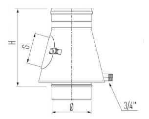
Inspection element with condensate drain - MEKI is part of the Schiedel ME range, which has a number of applications and advantages.
