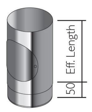
This item is used to provide Inspection and cleaning access. Available in 3 standard lengths - this is the shortest length.
