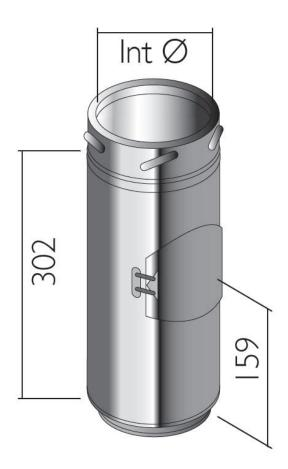
This article may be used as an aesthetic alternative to an Inspection tee on a connecting flue pipe system.
