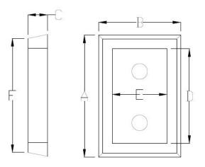
For Inspection Access. Suitable for use in negative pressure (Dry Chimney) applications. CE Designation (T450 N2 D 3 G)
