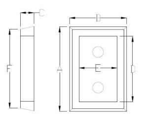
For Inspection Access. Suitable for use in negative pressure (Dry Chimney) applications. CE Designation (T450 N2 D 3 G)
